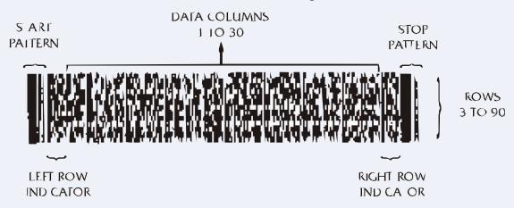
**Start and stop patterns** are used to delineate where a PDF417 begins and ends and makes reading symbol bi-directional.
