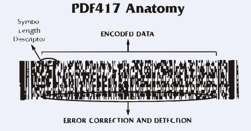
**Codewords** are the basic unit of storage in a PDF417 barcode. They contain data or error correction information and are used for row indicator information.
