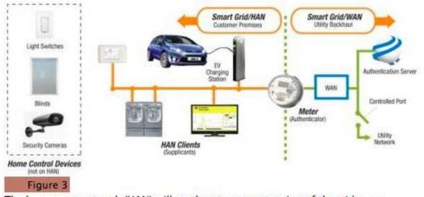
The home area network (HAN) will partly act as an extension of the wide area network (WAN) portion of the Smart Grid. In addition to smart metering, it will allow intelligent interaction with major appliances as well as electric vehicles.
